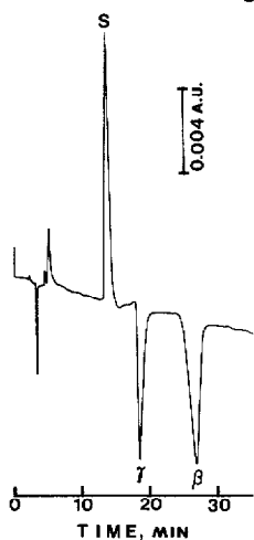
Fig. 1. Indirect photometric detection of cyclodextrins. Column: Develosil ODS-3K, 100 mm \times 0.35 mm I.D. Mobile phase: 0.3 mM phenolphthalein dissolved in 3% methanol solution, pH 12.2. Flow-rate: 2.8 \mu l/min. Samples: \beta = \beta -cyclodextrin; \gamma = \gamma -cyclodextrin; 2.0 mM of each was injected. Sample volume: 20 nl. Wavelength of detection: 550 nm.
